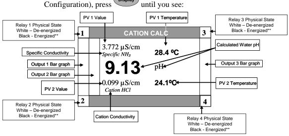
Figure 5-7 Cation Display screen example for pH calculations
